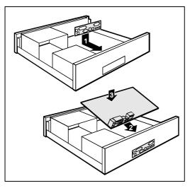
Should no suitable connection field be provided in the case, then you must install the connection field (1) provided.
